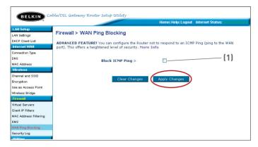
To turn off the ping response, select "Block ICMP Ping" (1) and click "Apply Changes". The Router will not respond to an ICMP ping.
